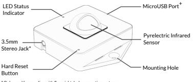
\* Only used for coupling with floorsight desk reservation systems \* Used to provide power for standalone floorsense systems
