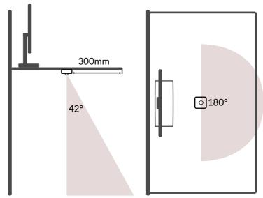
The range of detection is directly proportional to the height of the desk. For a desk equipped with adjustable height, the recommended distance from the front edge of the desk to the front of the module is 300mm. See Floorsen.se/ support for more information.
